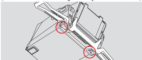
① Wrap the landing gear over the both sides of the battery footpads
