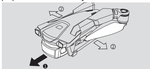
■ Press and hold the arm buttons until the arms are completely unfolded
