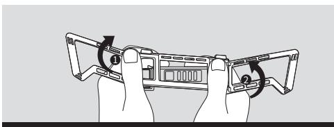
① Hold one side of the landing gear and push in the direction shown to remove it from the battery footpad
