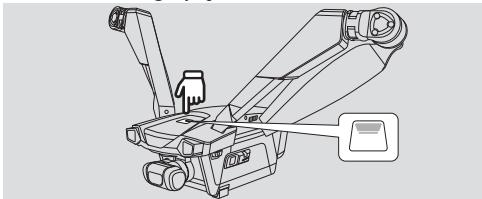
\* Note: There is no need to manually rotate the motors. The motor angle will automatically be in place before takeoff.
