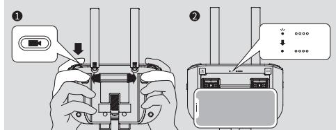
\* During the connection process, please keep the BlastOff Controller and the drone within 1 meter of each other.
