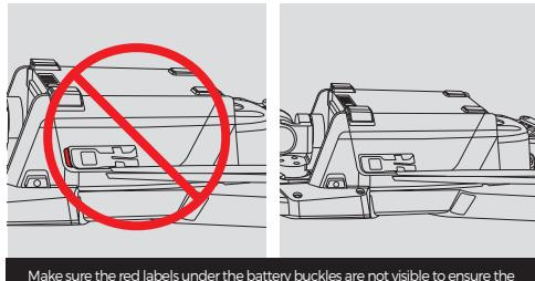
Make sure the red labels under the battery buckles are not visible to ensure the battery is securely installed
