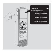
\* If the Hover 2 hotspot is not found, press and hold the Wi-Fi / RC toggle button on the drone for 4s, and try to connect again after hearing the beep.
